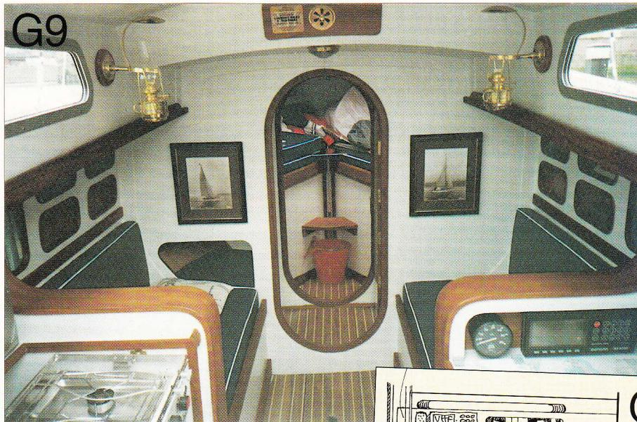
**G9** The finished interior. The quality of the work on the capping for the half-bulkhead can be seen here. It not only houses much of the navigation instrumentation, it provides an excuse to use a beautiful piece of teak on a lavish scale. On the bulkhead are two Beken photographs of the original *Vertue XXXV*, taken in 1950.
