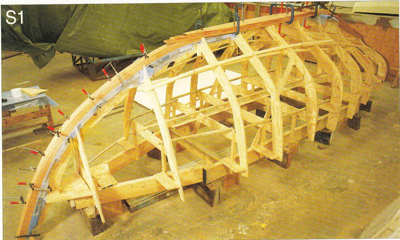
**C5** Decking. Once the planking is complete, the hull is braced and the internal moulds removed. The gunwale is then steamed and bent
